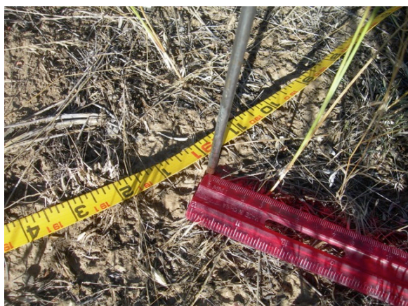
FIGURE 10: A visual of the line-point intercept method in action.
