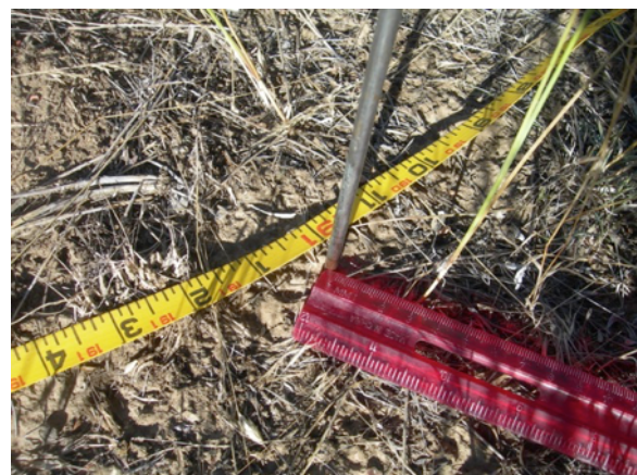
FIGURE 9: A visual of the line-point intercept method. The metal rod is lowered to the soil surface. Whatever it touches is recorded as “ground cover”. The ruler is used to measure the distance to the nearest perennial plant.
