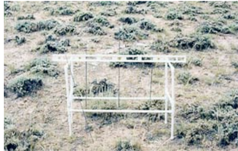
Figure 7: The point frame used in point intercept sampling for gathering ground cover and plant density data.
