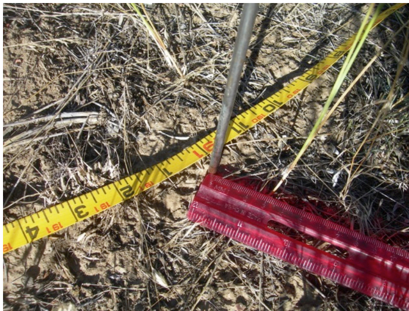
Figure 10: Utilizing the point intercept method to collect three quantitative measures of rangeland health. The steel rod is lowered to the soil surface to gather basal cover data. The distance to the nearest perennial plant is measured (in this case, a plant lies 3 cm from the rod) and that distance is averaged over 100 data points. Lastly, the nearest perennial plant's species is recorded (in this case, it is a Western wheatgrass).
